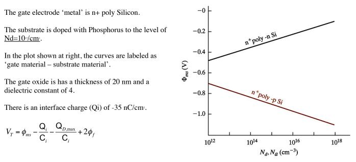
a) provide the value for how much the Fermi level in the substrate has been shifted from the intrinsic Fermi level due to doping (deeper into the substrate, where the bands are flat) [5 pts]:
